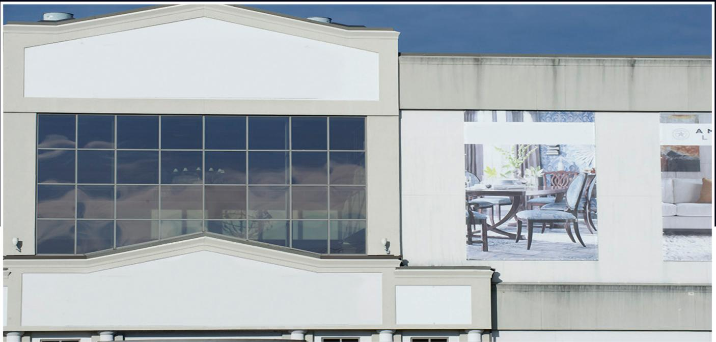
**Shown above:** The entire front face of this building was pressure washed. HDP Coating was applied to only the left portion of the building. Five years later, the left side is still clean while the right side is showing normal environmental conditions without HDP Coating.
