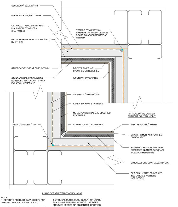
2. WALL ASSEMBLY SHALL PROVIDE FOR A MAXIMUM DESIGN DEFLECTION OF L/360.
