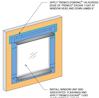
**INSTALL WINDOW UNIT AND** ASSOCIATED FLASHINGS AND APPLY TREMCO EXOAIR® 110AT OVER VERTICAL LEG OF FLASHING (SEE NOTE 1)
