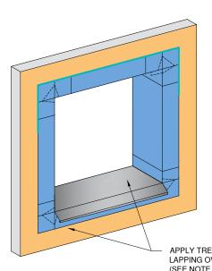
APPLY TREMCO EXOAIR® 110AT LAPPING OVER LIP OF SILL PAN FLASHING (SEE NOTE 1)
