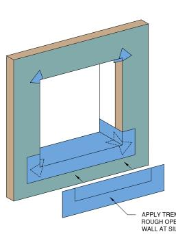
APPLY TREMCO DYMONIC® 100 ACROSS EDGE OF TREMCO® EXOAIR 110AT AT WINDOW HEAD AND DOWN JAMBS 6"
