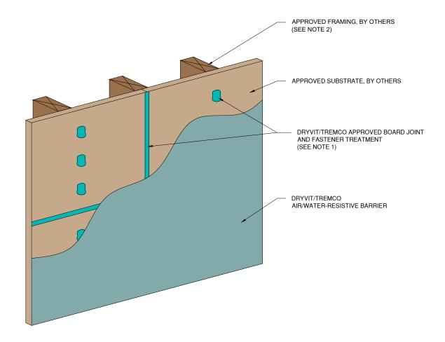
1. APPLY DYMONIC 100 ENSURING MINIMUM OVERLAP OF 3/4" (19 MM) ONTO EACH PANEL AT 40 MILS.
