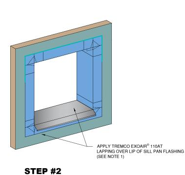
APPLY TREMCO DYMONIC® 100 ACROSS EDGE OF TREMCO® EXOAIR 110AT AT WINDOW HEAD AND DOWN JAMBS 6" INSTALL WINDOW UNIT AND ASSOCIATED FLASHINGS AND APPLY TREMCO EXOAIR® 110AT OVER VERTICAL LEG OF
