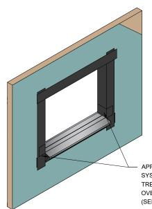
APPLY DRYVIT AQUAFLASH® SYSTEM OR TREMCO EXOAIR® 230 WITH TREMCO® 2011 MESH SPLICES LAPPING OVER LIP OF SILL PAN FLASHING. (SEE NOTE 1)
