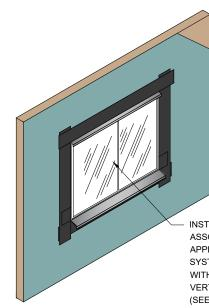
INSTALL WINDOW UNIT AND ASSOCIATED FLASHINGS AND APPLY DRYVIT AQUAFLASH SYSTEM OR TREMCO EXOAIR 230 WITH TREMCO 2011 MESH OVER VERTICAL LEG OF FLASHING (SEE NOTE 1)
