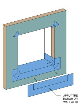
APPLY TREMCO EXOAIR® 110AT 3" MIN INTO ROUGH OPENING AND EXTERIOR FACE OF WALL AT SILLS, JAMBS AND HEADS
