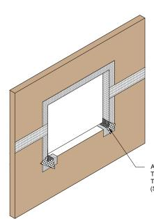
APPLY DRYVIT GRID TAPE™ OR TREMCO EXOAIR® 230 WITH TREMCO® 2011 MESH (SEE NOTES 1, 2, 5)
