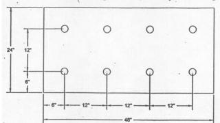
Pattern "C" - For use with structural substrates such as: wood sheathing, concrete, masonry, metal siding
