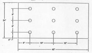
Pattern "D" - For use with structural substrates such as:
